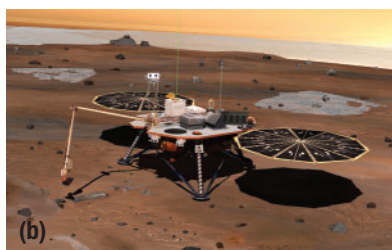
Figure 1 (a) A scientist in a “clean room” makes final adjustments to the Thermal and Evolved Gas Analyzer (TEGA) that the Phoenix used to detect water and organic compounds. (b) An artist’s impression shows the robotic arm of the Phoenix (lower left) about to take a soil sample.
