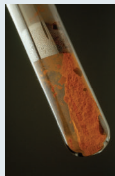
Figure 3 Heating a compound of mercury and oxygen leaves a mirror-like coating of mercury lining the test tube.
