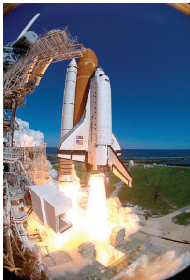
Figure 1 The combustion of hydrogen fuel was used to launch the space shuttle into orbit. Aboard the shuttle, hydrogen fuel cells used the same chemical reaction to provide astronauts with electricity and water.
