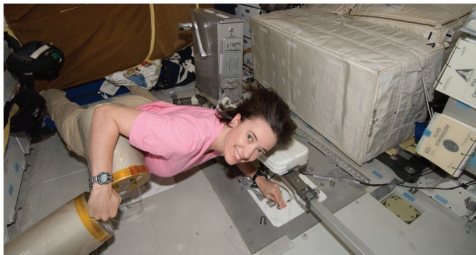
Figure 1 An astronaut changes a lithium hydroxide canister used to scrub carbon dioxide from the interior air during space missions. Each canister lasts about 11 hours for a seven-person crew.
