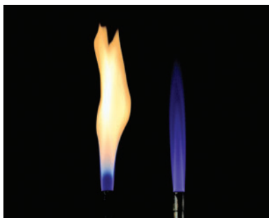
Figure 1 When you light a Bunsen burner, you start with an orange flame then adjust the air intake to get a hot, blue flame.
