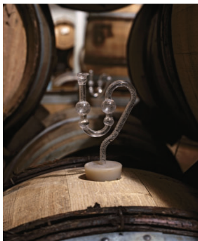
Figure 1 Fermentation locks filled with water are fitted to the top of each bottle, allowing carbon dioxide to escape while preventing oxygen from entering. If the bottles were sealed, the pressure from the accumulating carbon dioxide could break them.
