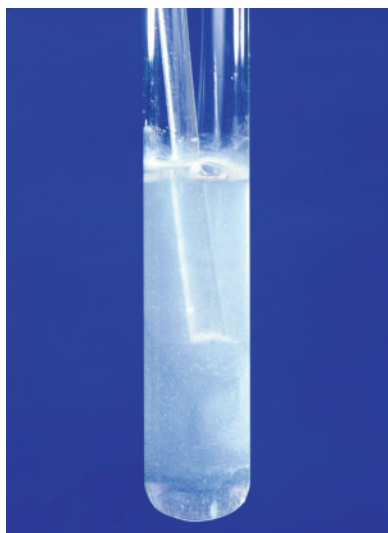
Figure 5 When carbon dioxide bubbles through a straw into a solution of calcium hydroxide (limewater), a precipitate turns the liquid cloudy. This reaction is used in the familiar limewater test for carbon dioxide.
