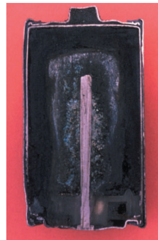
Figure 3 The fluid paste in an alkaline cell must be a good conductor of electricity in order for the cell to generate electricity. These cells are called “alkaline” because they contain the base potassium hydroxide, KOH.
