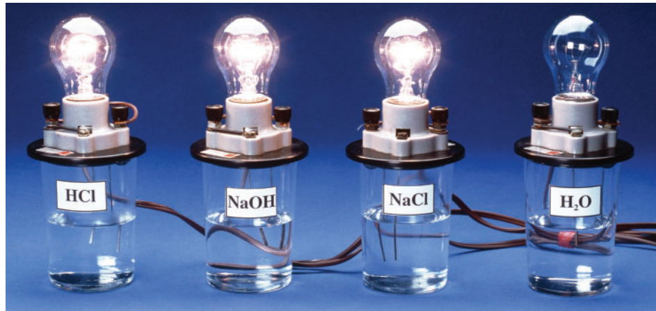
Figure 1 Solutions of hydrochloric acid, sodium hydroxide, and sodium chloride are good conductors of electricity because of the ions they contain. According to Arrhenius, pure water is a poor conductor because it does not contain ions.
