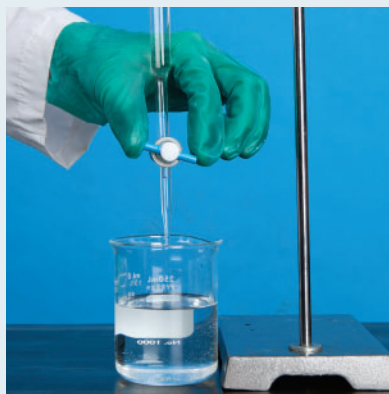
Figure 8 Air bubbles in the tip and valve must be cleared before starting a titration.
