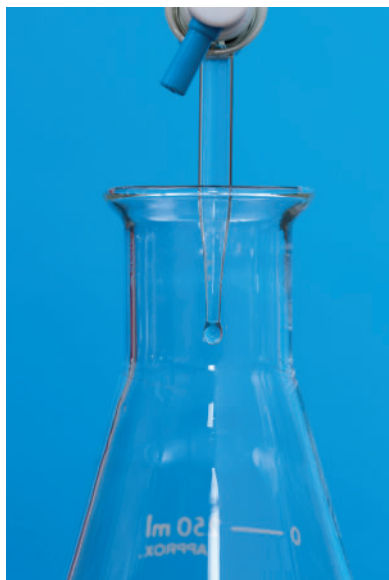
Figure 10 The burette tip should remain in the flask throughout the titration.
