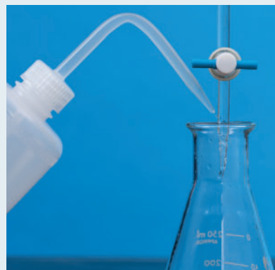
Figure 12 Rinse the tip and sides of the titration flask with distilled water prior to the endpoint.
