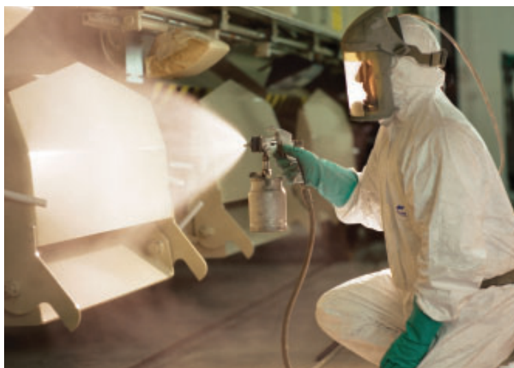
Figure 12 Curved objects and objects with open spaces (such as fencing) are often painted using an electrostatic paint sprayer. The attraction of the paint particles to the oppositely charged object ensures that paint will wrap around the curved portions of the object, rather than fall through the open spaces.
