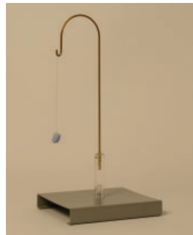
Figure 5 A pith ball electroscope is a simple device that can be used to detect the presence of electric charges.
