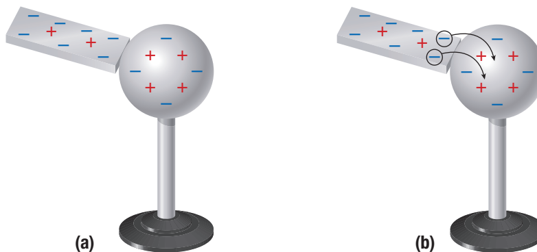
Figure 4 A neutral metal sphere (a) becomes charged by conduction when brought in contact with a negatively charged bar. Some of the electrons are transferred from the bar to the sphere, resulting in an overall negative charge on the sphere (b).
