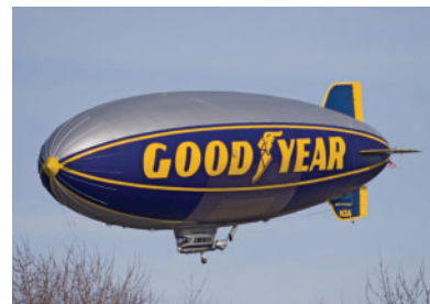
Figure 2 Blimps generate lift by using gases that are lighter than air. Although hydrogen is lighter than helium, it is no longer used because it is flammable.
