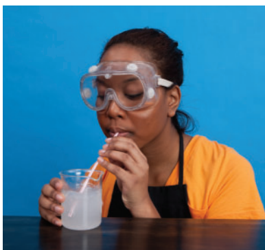
Figure 4 Always blow out through limewater.
