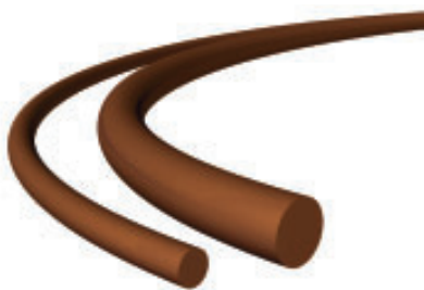
Figure 1 The wire at the left has a smaller diameter cross-section than the wire at the right. The thinner wire will have more internal resistance than the thicker wire.
