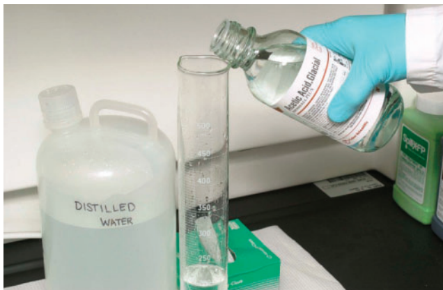
Figure 1 Steam forms when concentrated acid is added to water. When diluting acids, always add acid to water.
